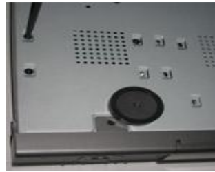
Fig 2-2 Screw HDD
